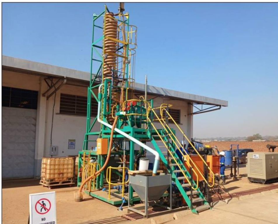
Figure 95: Installed Spiral plant at Sovereign's Lilongwe facility.
