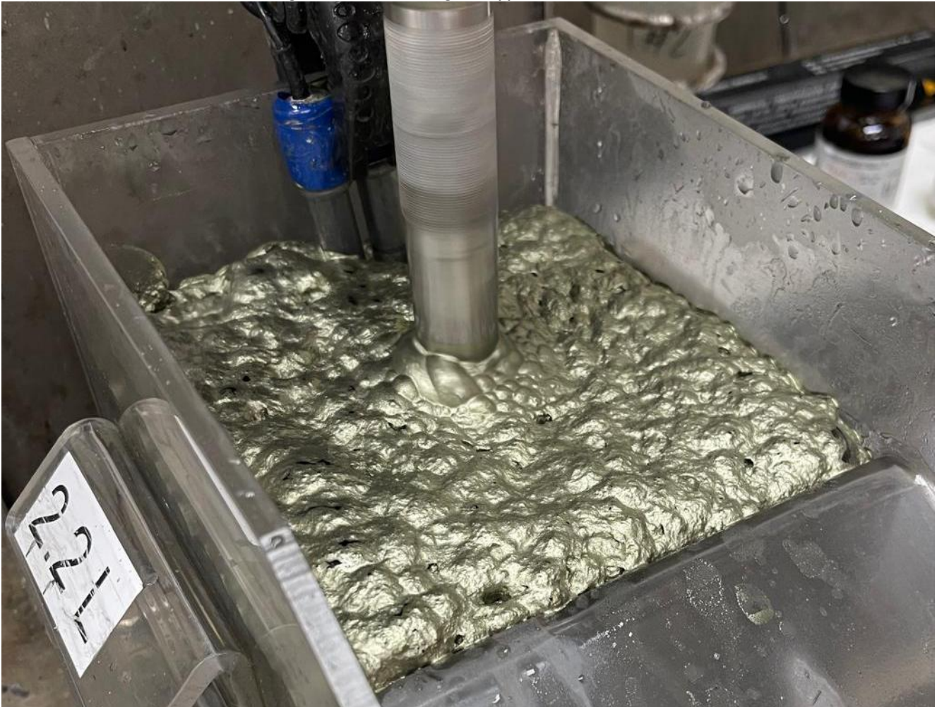
Figure 5 – Boi Novo Rougher Copper-Gold Concentrate
