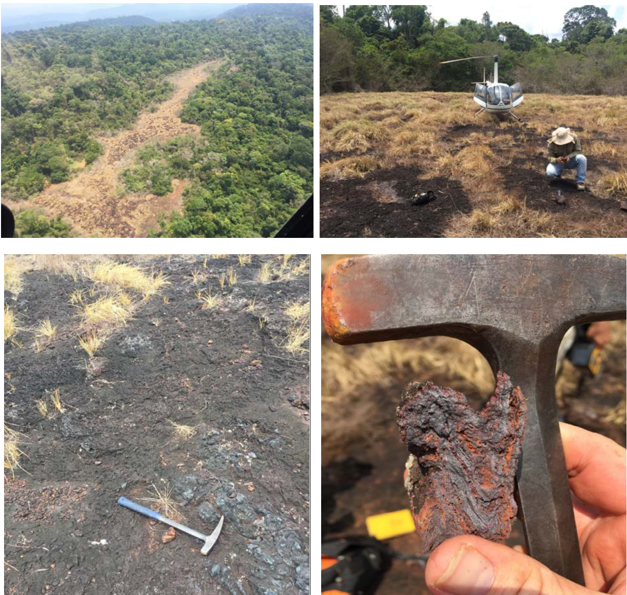
Figure 1 – Canga Prospect (clockwise from top left: aerial view of Canga Prospect from ENE; Centaurus Senior Geologist Gaudius Montresor inspects the outcrop; small fold shows original bedding; massive hematite zones within the lateritized iron formation)
