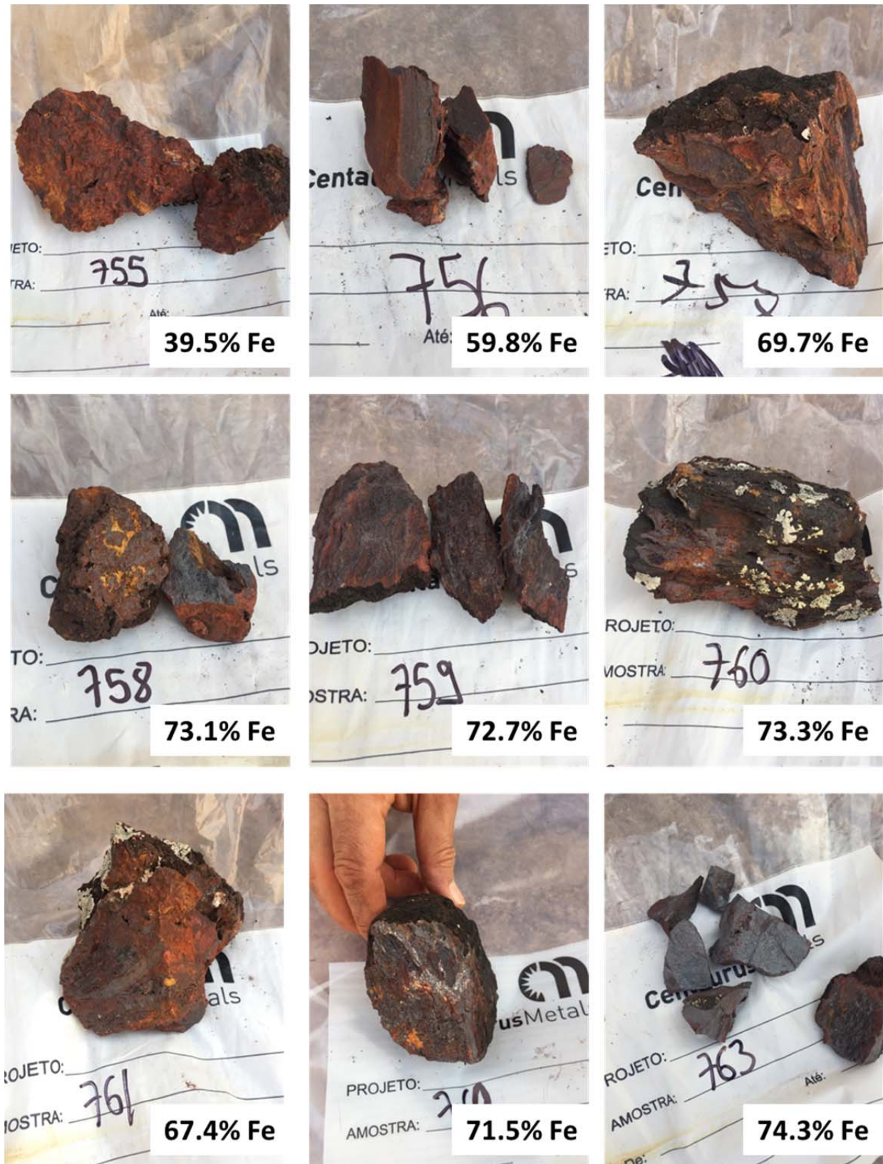
Figure 3 – Rock chip samples taken from Canga Outcrop (Fe grade from hand held Olympus Delta XRF)
