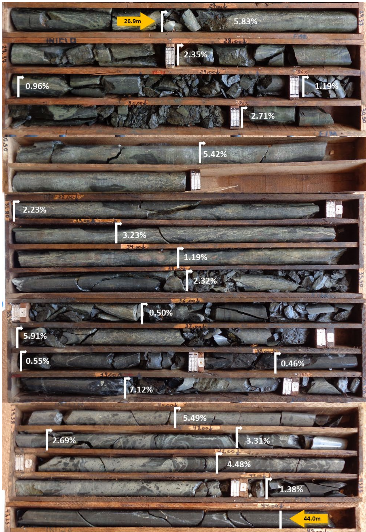
Figure 7 – Core photos from drill hole JAG-DD-20-029; 26.9 to 44.0m: Semi-massive and massive sulphides (metallic bronze/yellow colour) with magnetite (black colour) mineralisation hosted in altered dacite. Sulphides comprising pyrite, pentlandite, millerite, violarite, minor chalcopyrite and sphalerite. This interval returned 16.1m at 3.07% Ni, 0.14% Cu and 0.07% Co from 26.9m.
