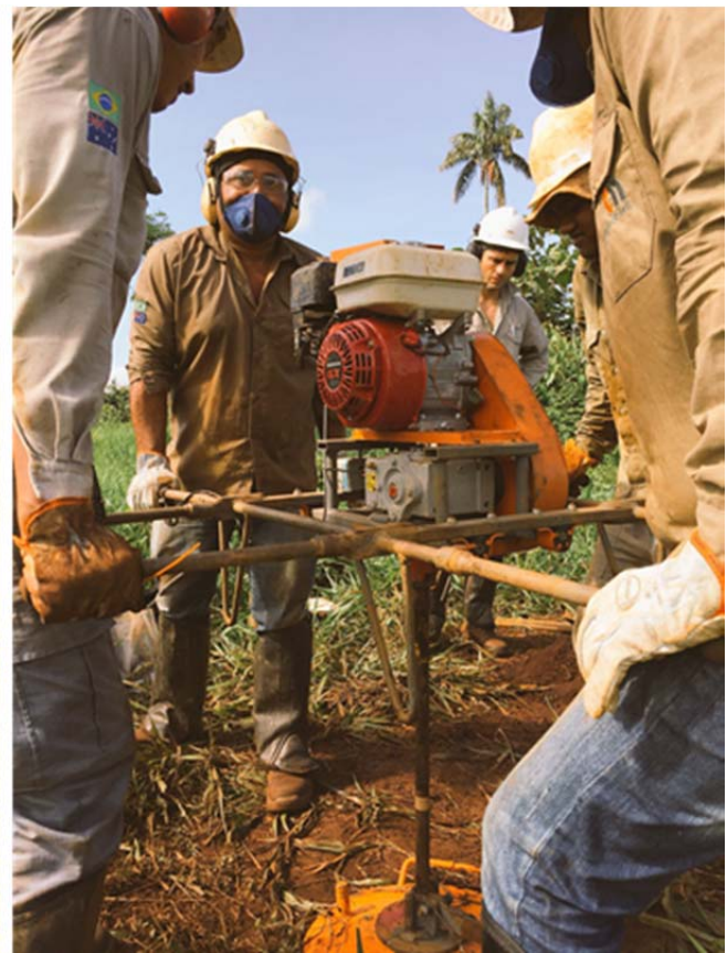
Figure 4 – Photos of the auger drilling at the Itapitanga Ni-Co Project; Moving hole (left), field team work hard to secure the new auger drill (right).
