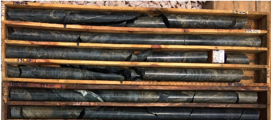
Figure 8 – Core photos from drill hole JAG-DD-19-001; 126.1 to 129.0m returned 2.9m at 3.80% Ni: Visual estimates of the interval was described as semi-massive and massive sulphides with intense magnetite mineralisation - 30-40% sulphides comprising py, pn, mlr, cp, sp;
