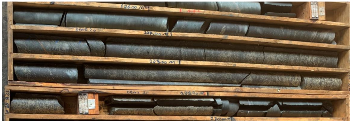
Figure 8 – Core photos from drill hole JAG-DD-19-001; 126.1 to 129.0m returned 2.9m at 3.80% Ni: Visual estimates of the interval was described as semi-massive and massive sulphides with intense magnetite mineralisation - 30-40% sulphides comprising py, pn, mlr, cp, sp;
