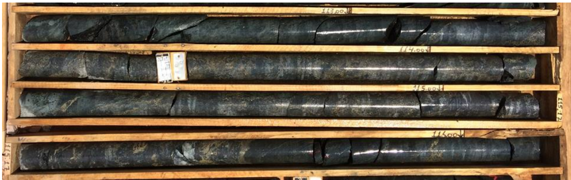
Figure 6 – Core photos from drill hole JAG-DD-19-002; 113.00m to 115.75m returned 2.5m at 3.38% Ni; Visual estimates of the interval were described as semi-massive and massive sulphides with intense magnetite mineralisation - 10-20% sulphides comprising mlr, pn, py, cp, po 1
