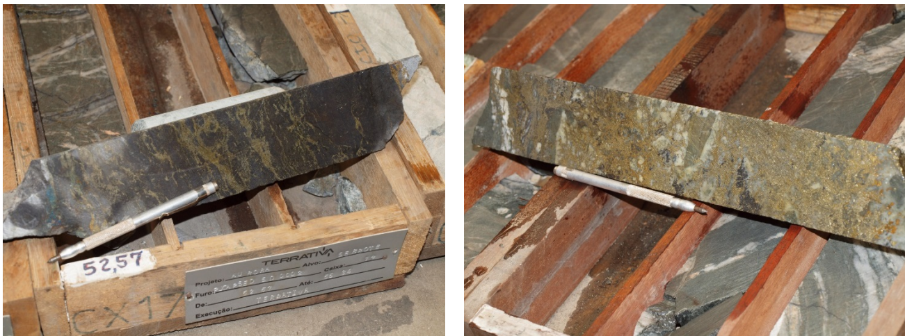
Figure 5: Left - Terrativa DDH PJCA-PSED-SD0002 (50.0-53.9 metres – 1.08% Cu); Right - Terrativa DDH PJCA-PSED-SD0004 (109.0-110.0 metres – 2.13% Cu)
