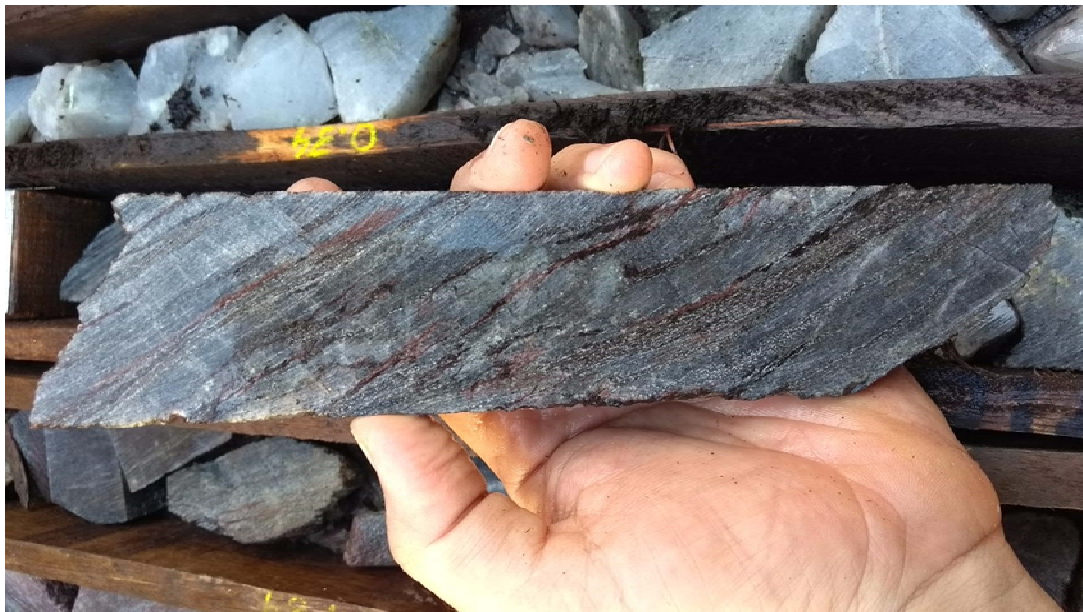
Figure 3: SRM-DD-17-002 intersected a hydrothermal breccia with silica and muscovite alteration plus sulphides (6m at 0.7g/t Au from 84m, including 2m at 1.4 g/t Au; photo: 84.3m – 1.8g/t Au)
