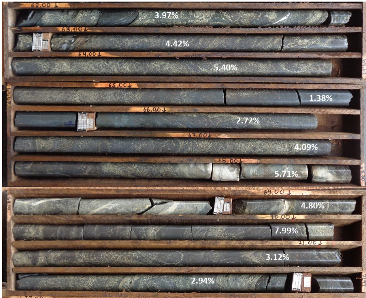
Figure 5 – Core photos from drill hole JAG-DD-20-021; 62.0 to 72.3m: Semi-massive and massive sulphides (metallic bronze/yellow colour) with intense magnetite (black colour) mineralisation - 10-40% sulphides comprising pyrite, pentlandite, millerite, chalcocopyrite and sphalerite. This interval returned 9.6m at 4.19% Ni, 0.29% Cu and 0.16% Co from 62.3m.
