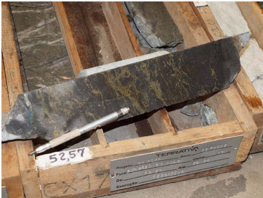
Figure 5 – Aurora Project – Terrativa DDH PJCA-PSED-SD0002 (50.0-53.9 metres - 1.08% Cu)
