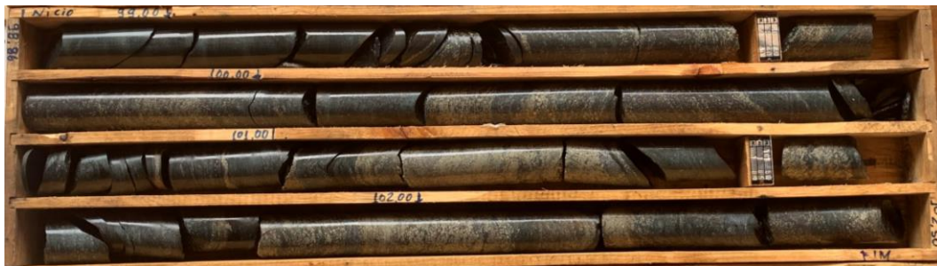
Figure 6 – Core photos from drill hole JAG-DD-19-003; 99.2m to 102.8m: 3.6m of semi-massive and massive sulphides with intense magnetite mineralisation - 30-40% sulphides comprising py, pn, mlr, cp, sp
