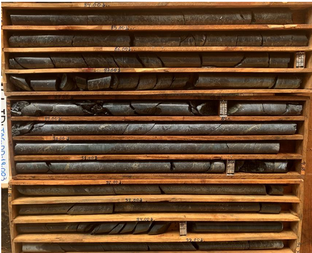
Figure 12 – Core photos from drill hole JAG-DD-19-003; 83.6 to 89.4m: 5.8m semi-massive and massive sulphides with intense magnetite mineralisation - 5-10% sulphides comprising py, pn, mlr, po, cp; and 89.2m to 95.7m: 6.5m of semi-massive and massive sulphides with intense magnetite mineralisation - 30-40% sulphides comprising py, pn, mlr, cp, sp
