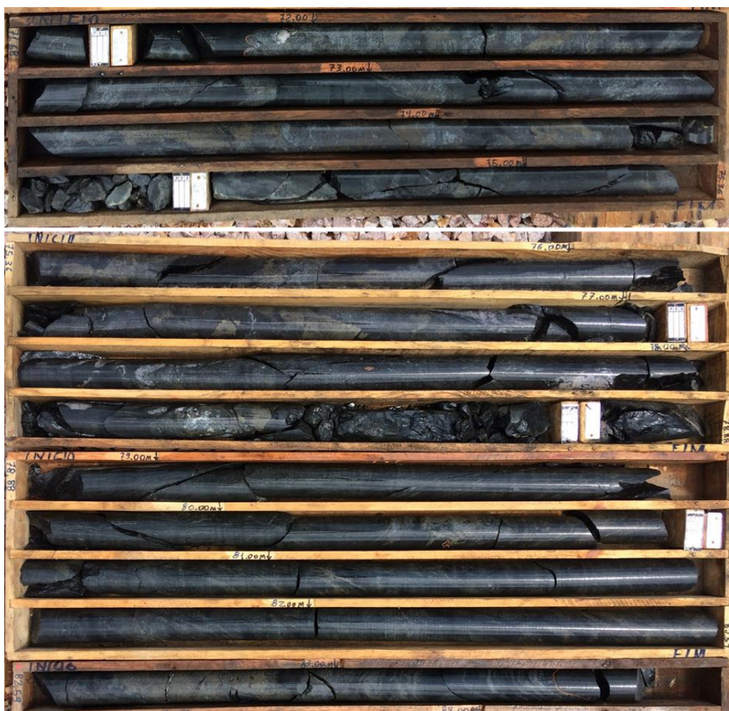
Figure 3 – Core photos from drill hole JAG-DD-19-002; 72.00m to 83.40m: 11.40m of semi-massive and massive sulphides with moderate to intense magnetite mineralisation - 10-20% sulphides comprising mlr, pn, py, cp, po.
