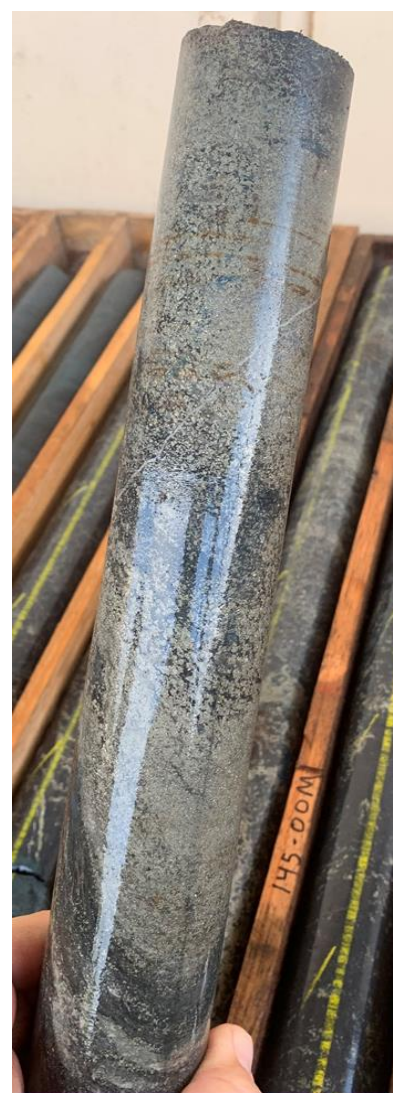
JAG-DD-19-001 – semi-massive and massive sulphides at 146.15m.
