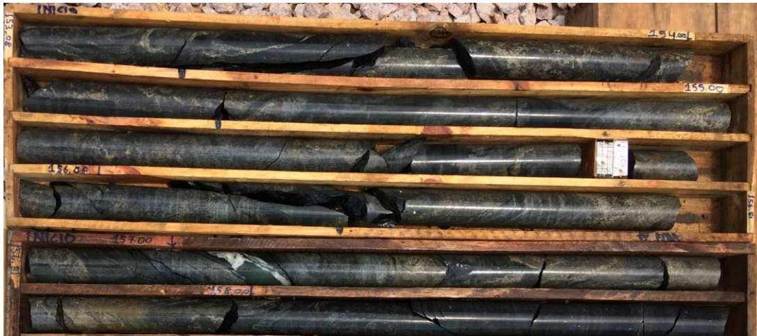
Figure 9 – Core photos from drill hole JAG-DD-19-002; 153.0m to 158.05m: 5.05m of semi-massive and massive sulphides with intense magnetite mineralisation - 10-20% sulphides comprising mlr, pn, py, cp, po
