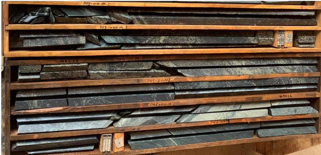
Figure 12 – Core photos from drill hole JAG-DD-19-003; 83.6 to 89.4m: 5.8m semi-massive and massive sulphides with intense magnetite mineralisation - 5-10% sulphides comprising py, pn, mlr, po, cp; and 89.2m to 95.7m: 6.5m of semi-massive and massive sulphides with intense magnetite mineralisation - 30-40% sulphides comprising py, pn, mlr, cp, sp
