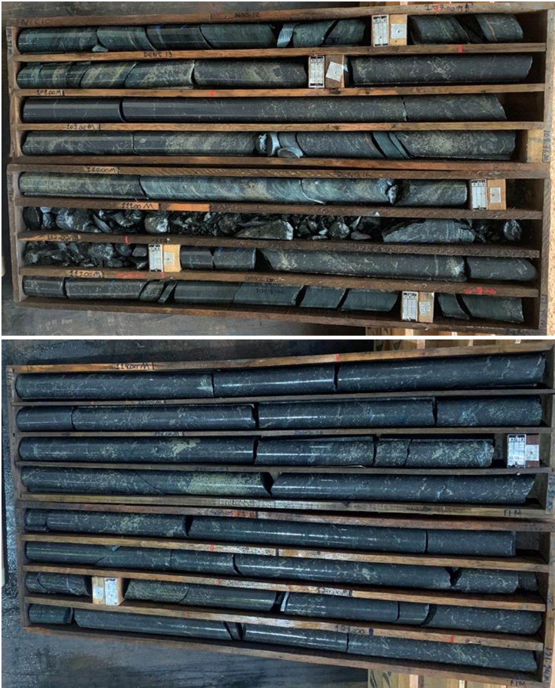
Figure 10 – Core photos from drill hole JAG-DD-19-001; 106.95 to 112.10m: 5.15m of semi-massive and massive sulphides with intense magnetite mineralisation - 10-20% sulphides comprising py, pn, mlr, cp, sp; and 112.1 to 121.0m; 8.9m of stringer and semi-massive sulphides with intense magnetite mineralisation - 5-10% sulphides comprising py, pn, mlr, po.
