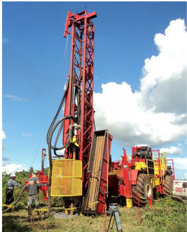
Figure 4 – Photo of the hand-held auger working at the Itapitanga Ni-Co Project (left) versus the RC drill rig that is now operating on site (right);
