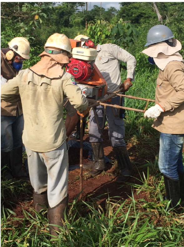
Figure 4 – Photo of the hand-held auger working at the Itapitanga Ni-Co Project (left) versus the RC drill rig that is now operating on site (right);
