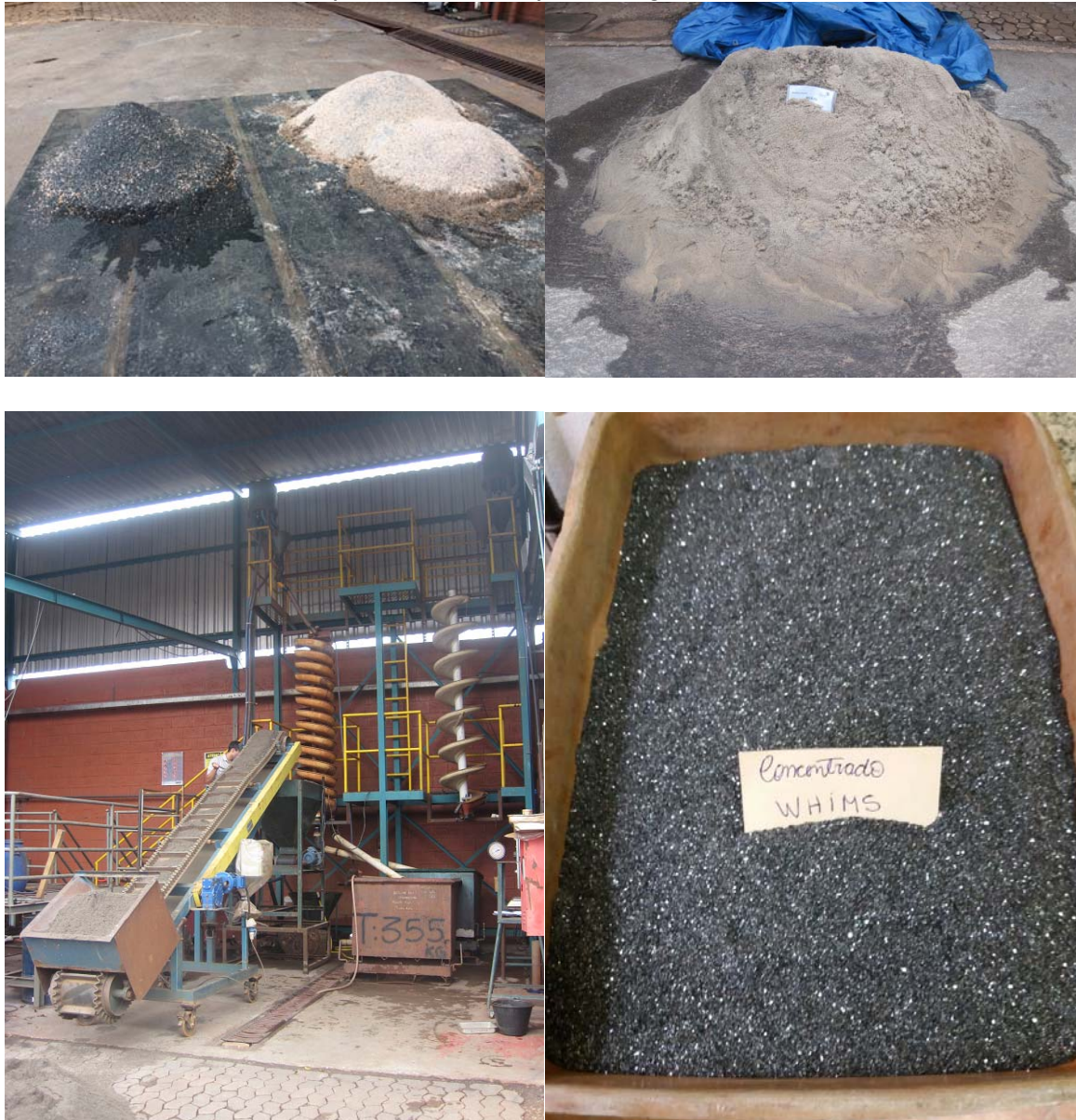
Figure 1 – Top Left – Jig Concentrate and Jig Tails; Top Right – Spirals Tailings Bottom Left – Spirals Testwork Facility; Bottom Right – WHIMS Concentrate.
