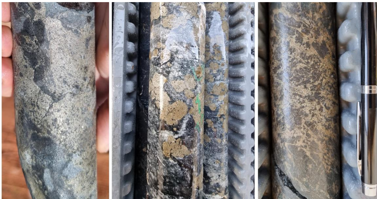
Figure 5 (A) volcanic-hosted massive sulfide, (B) blebby sulfide, and (C) breccia-texture sulphides
