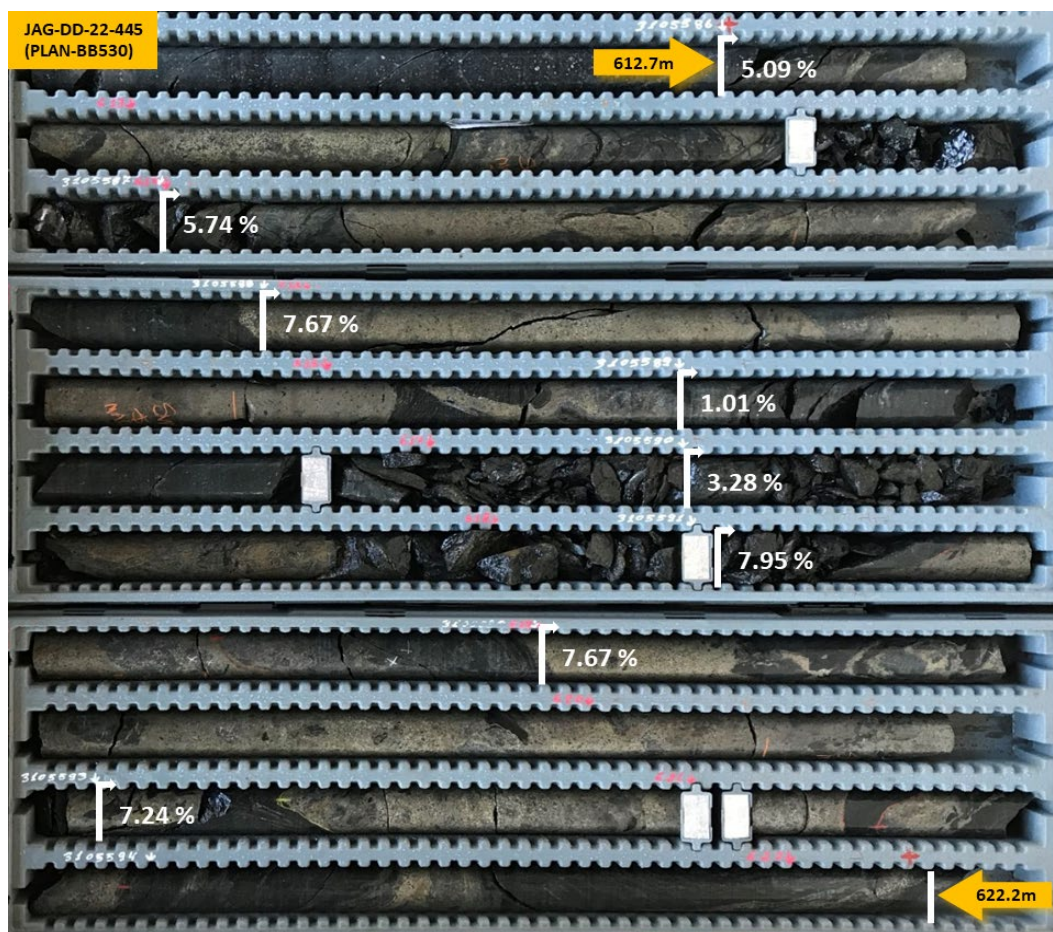
Figure 1 – The Jaguar South Deposit: Core photo from drill-hole JAG-DD-22-445 from 612.7m which returned 9.5m at 5.59% Ni down-hole, including stringer, semi-massive and massive sulphides (dark metallic bronze) mineralisation with altered dacite host rock.
