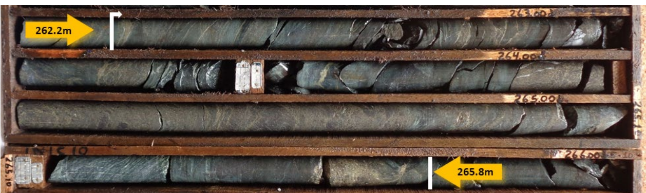
Figure 12 – Core photos from drill hole JAG-DD-20-45 (Onça Rosa); 262.2 to 265.8.3m: Semi-massive to massive sulphides (metallic bronze/yellow colour) with intense magnetite (black colour) mineralisation hosted in altered granite. Sulphides comprising pyrite, pentlandite, millerite and minor chalcopyrite. Assays awaited
