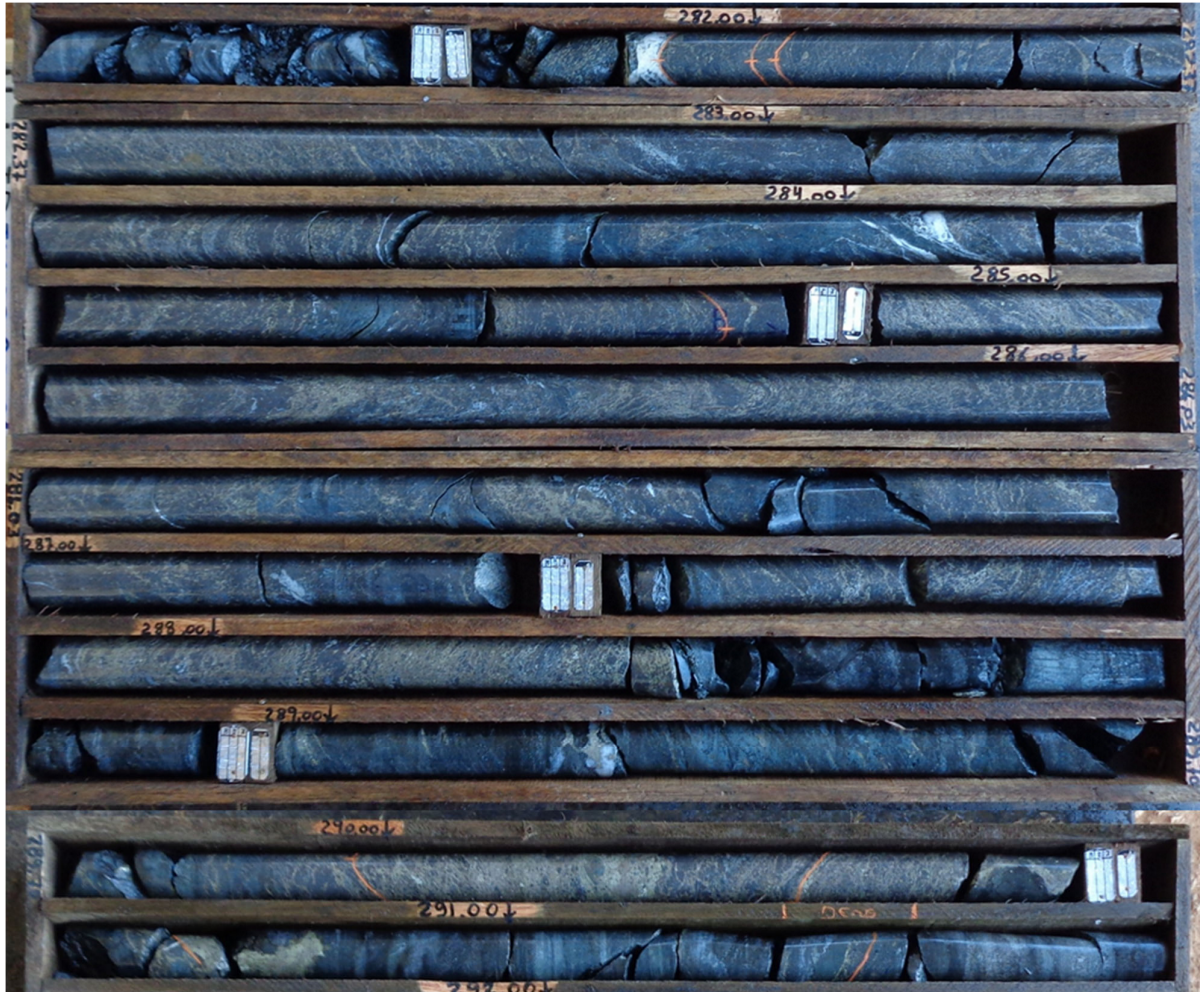
Figure 4 – Core from drill hole JAG-DD-19-017; 281.75 to 291.1m: 9.35m of semi-massive and massive sulphides with intense magnetite mineralisation - 10-30% sulphides comprising pyrite, pentlandite, millerite, chalcocpyrite and sphalerite. This interval returned 9.3m at 3.13% Ni, 0.19% Cu and 0.08% Co.
