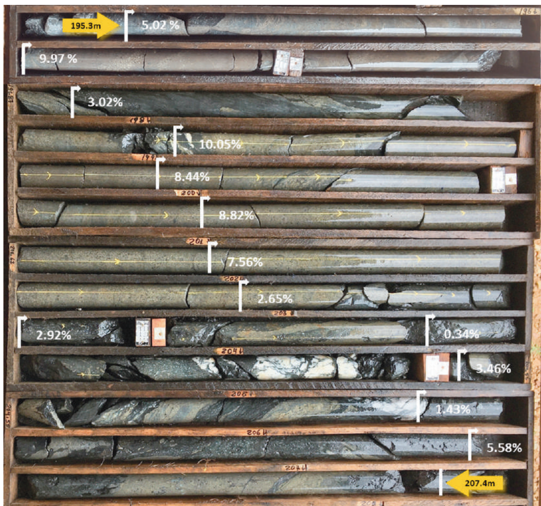
Figure 5 - Core photo from drill hole JAG-DD-20-104, 195.3m to 207.4m for 12.1m at 5.38% Ni, 0.31% Cu and 0.09% Co.
