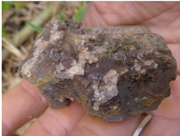
Figure 2 – Quartz vein with Limonite pseudomorphs after pyrite with boxworks (674377mE, 7851107mN).
