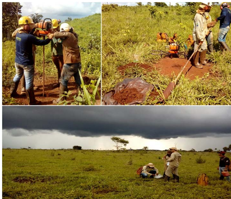
Figure 5 – Photos of the auger drilling at the Itapitanga Ni-Co Project; Four-man hand held auger (top left), removing the sample from auger bit (top right), working to beat the afternoon rain (bottom).
