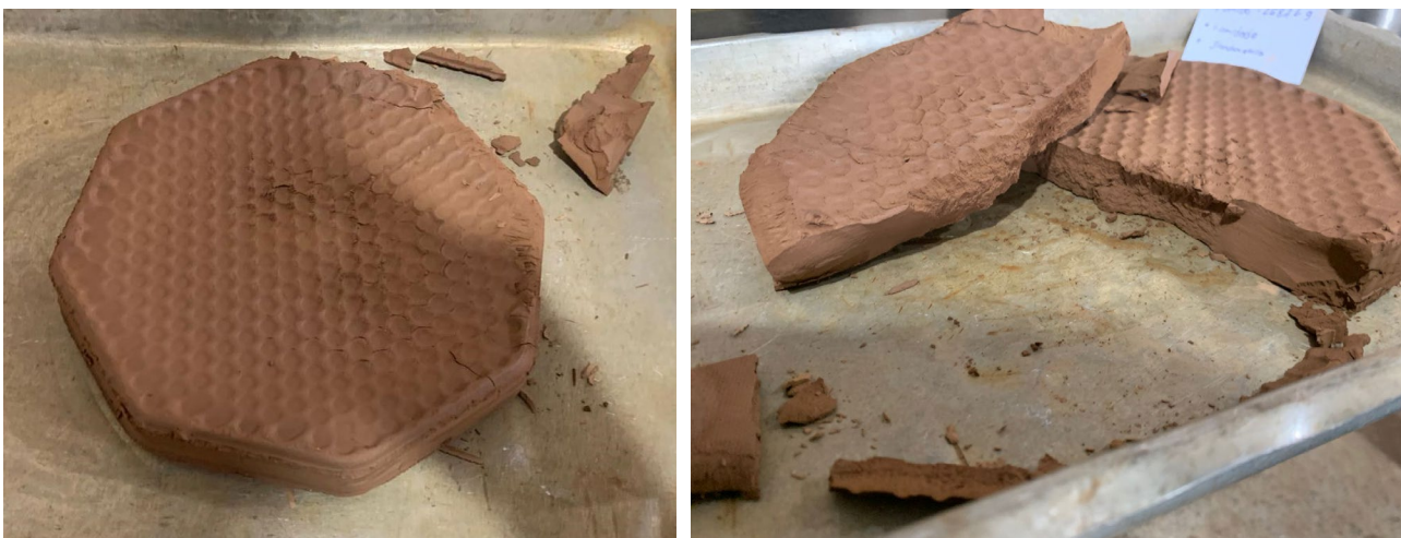
Figure 3 – Jambreiro Filtered Tailings Cake
