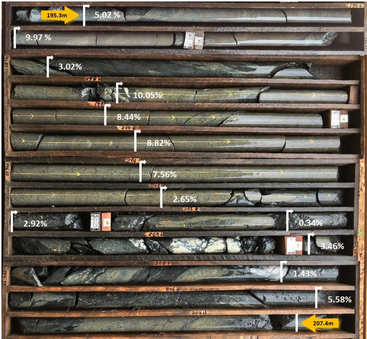
Figure 4 – Core photo from drill hole JAG-DD-20-104 (Jaguar Central); 195.3m to 207.4m down-hole: Stringer to semi-massive and massive sulphides (metallic bronze/yellow colour) with magnetite (black colour) mineralisation hosted in altered dacite. This interval returned: 12.1m at 5.38% Ni , 0.31% Cu and 0.09% Co from 195.3m.
