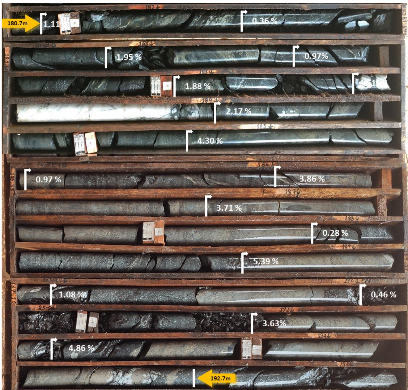
Figure 3 – Core photo from drill hole JAG-DD-20-104 (Jaguar Central); 180.7m to 192.6m down-hole: Stringer to semi-massive and massive sulphides (metallic bronze/yellow colour) with magnetite (black colour) mineralisation hosted in altered dacite. This interval returned: 12.0m at 2.31% Ni , 0.21% Cu and 0.05% Co.
